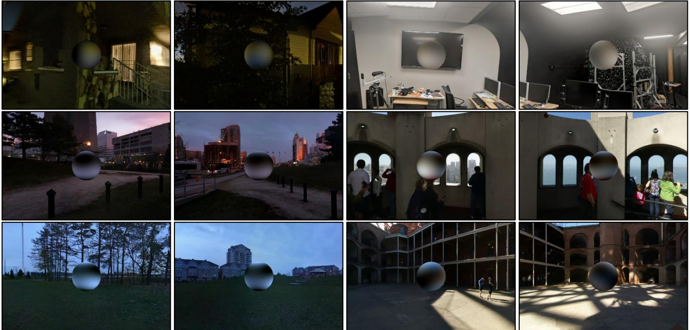
Fig. 1. Above are pictures of final rendering outputs, we can compare these pictures pair by pair (left to right). Based on SH method, our light engine can render the loaded sphere model successfully. We can see the lights projected on the surface of the sphere, and they will change when we rotate the environment.
